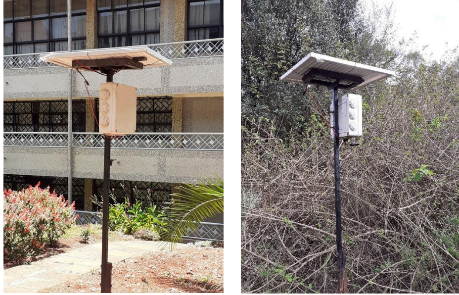
Figure 8: DSAIL Bioacoustics System deployment outside the university Resource Centre for power analysis of the system (left) and at the university conservancy to collect acoustic data of birds (right).
