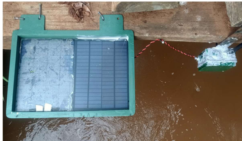
Water Level sensor
